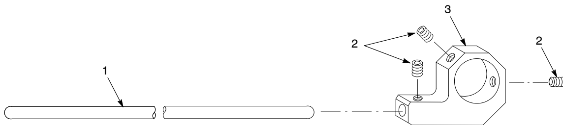
Figure 7-5 Shur-Lok Mount Ion Collector Kit
