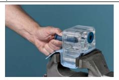
Pull the pinch valve firmly until it comes out of the pinch valve body.
