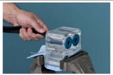
Pull the pinch valve insertion tool firmly until the UP end of the pinch valve and the entire insertion tool come out the top of the pinch valve body.
