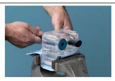
Turn the pinch valve body around so that the top end faces you. Insert the pinch valve insertion tool into the pinch valve body.
