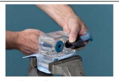
Insert the UP end of the pinch valve into the pinch valve insertion tool. Pinch the UP end and feed the small end into the pinch valve body.
