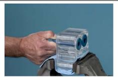
Place the pinch valve body in a padded vise with the bottom end facing you. Grasp and pull the bottom end of the pinch valve with one hand.
