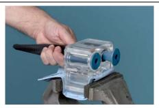
While pinching the UP end of the pinch valve in the insertion tool, pull the insertion tool.
