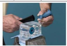
**NOTE:** After you put the pinch valve into the insertion tool, pinch the UP end of the valve.
