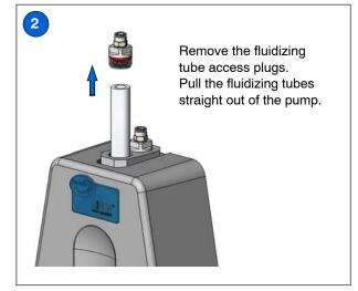
Check the O-rings in the inside diameter of the access plugs. Replace them if necessary.
