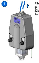
Shut off and relieve the purge air pressure. Disconnect the purge air tubing.
