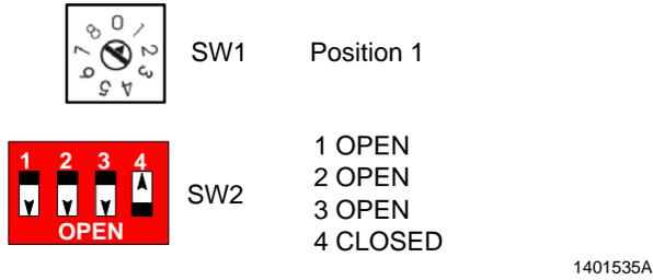
Figure 4 SW1 and SW2 Settings for a Manual Powder Spray Systems
