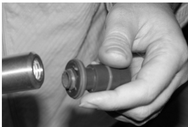
Figure 7 Nozzle Disassembly Step 3 (New Style Shown)
