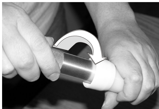
Figure 5 Nozzle Disassembly Step 2A
