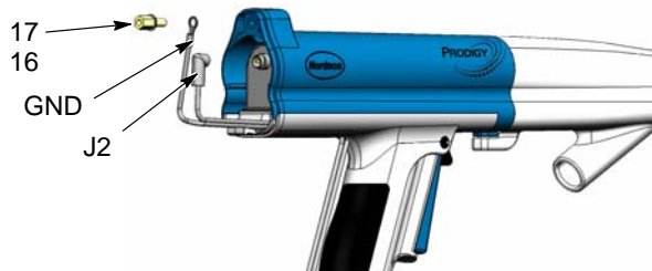
Figure 19 Disconnecting the Control Cable
