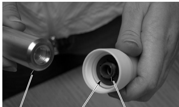
Figure 4 Nozzle Disassembly Step 1 (Shown with Nut Installed)
