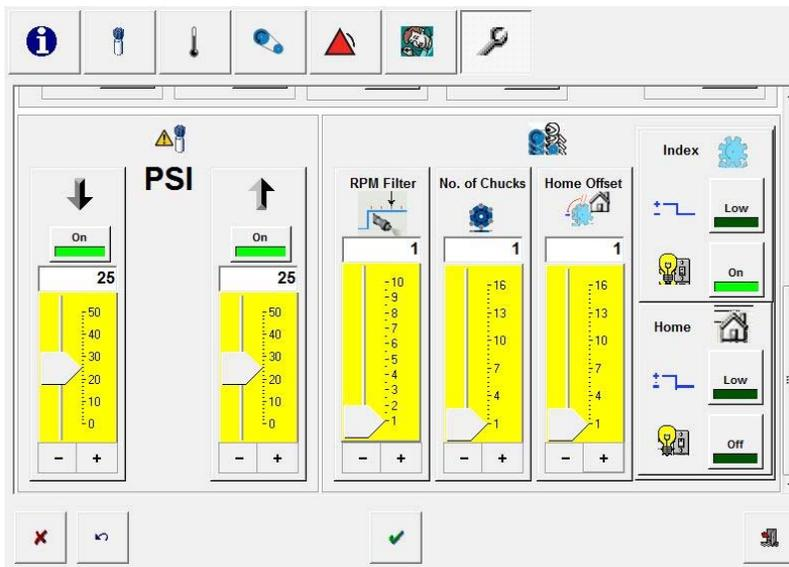
7. Enter a value for the **RPM Filter**. This prevents the chuck speed from being read until the chuck is up to speed. For example, if the spray duration is 100 milliseconds, and the system sees 10 speed targets during that time, a setting of 5 will cause the system to wait until the 5th target is sensed before reading the chuck speed. For a better explanation, see this diagram.
