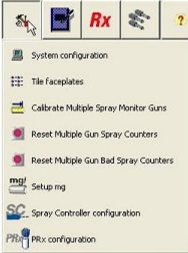
2. Touch **Calibrate Multiple Spray Monitor Guns** and calibrate the Spray Monitors for which you want to monitor mg weight. Weigh the cans coated during the calibration procedure and calculate the average weight applied. If the applied weight is not satisfactory, adjust your system to obtain the desired coating weight and calibrate again.
