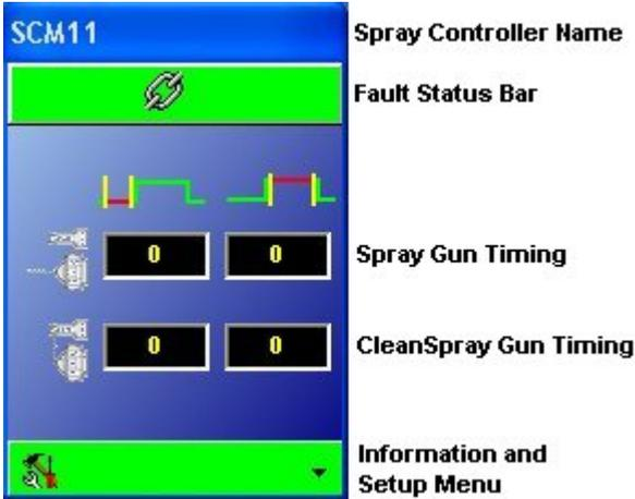
The fault status bar and the information and setup bar are green during normal operation. They change to yellow when a warning occurs and red when an alarm occurs.
