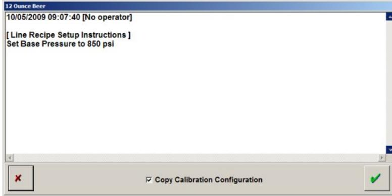
4. By default, the Spray Monitor Calibration Configuration settings and Calibration Data are copied to the modules when the recipe is loaded. If you do not want this to happen, touch the **Copy Calibration Configuration checkbox** to de-select it.
