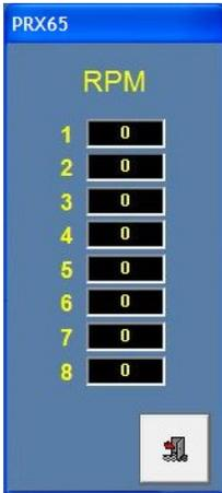
Depending on the configuration, this window will either show the speed of the current chuck, or the last speed measured of all the chucks on the turret.
