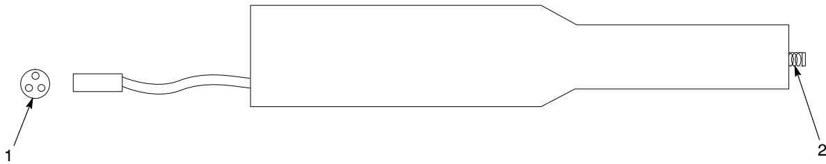
Figure 6-8 Multiplier Continuity and Resistance Check
