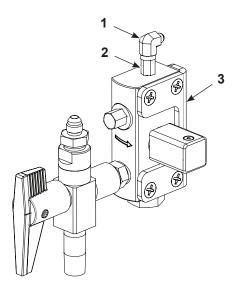
Figure 1 ezSPC manifold with Retrofit Fittings
