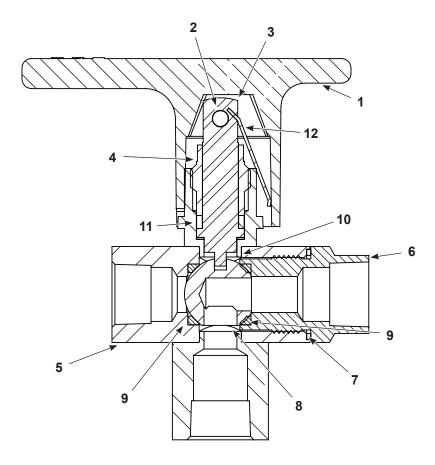
Figure 1 3-way Ball Valve Assembly
