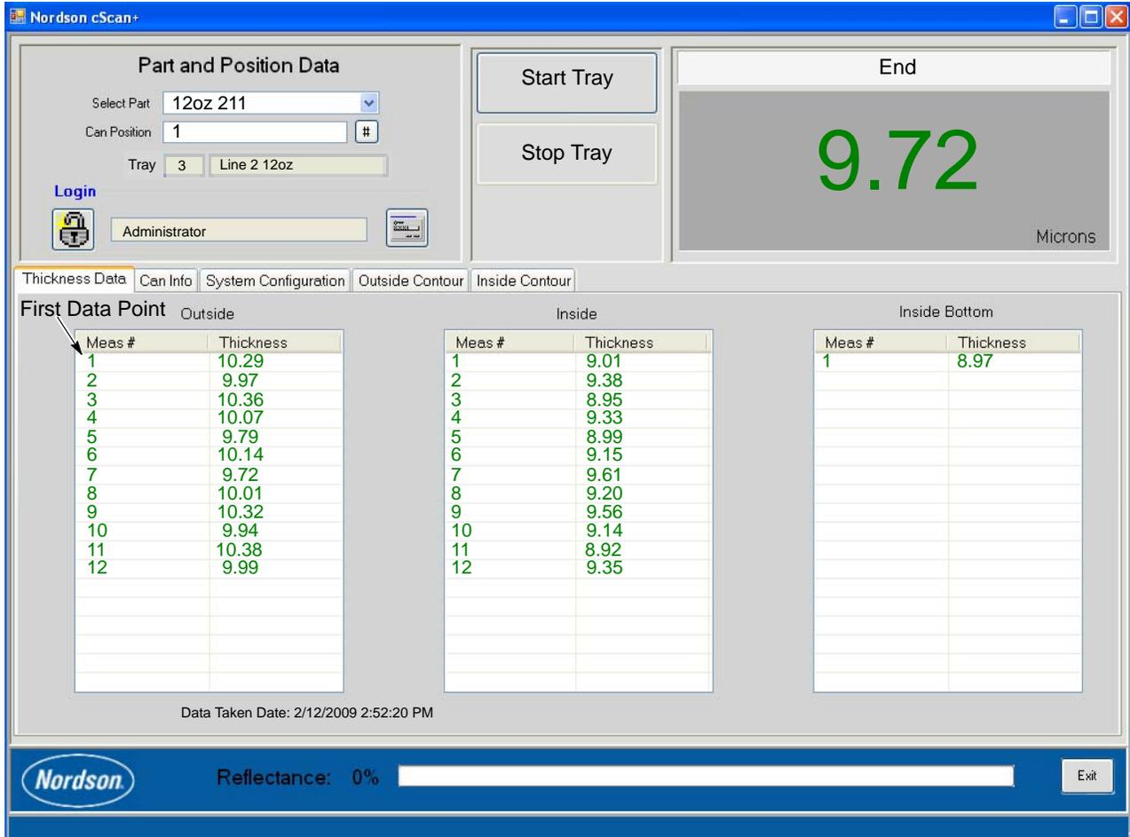
Figure 34 Measurements from Thickness Data Screen
