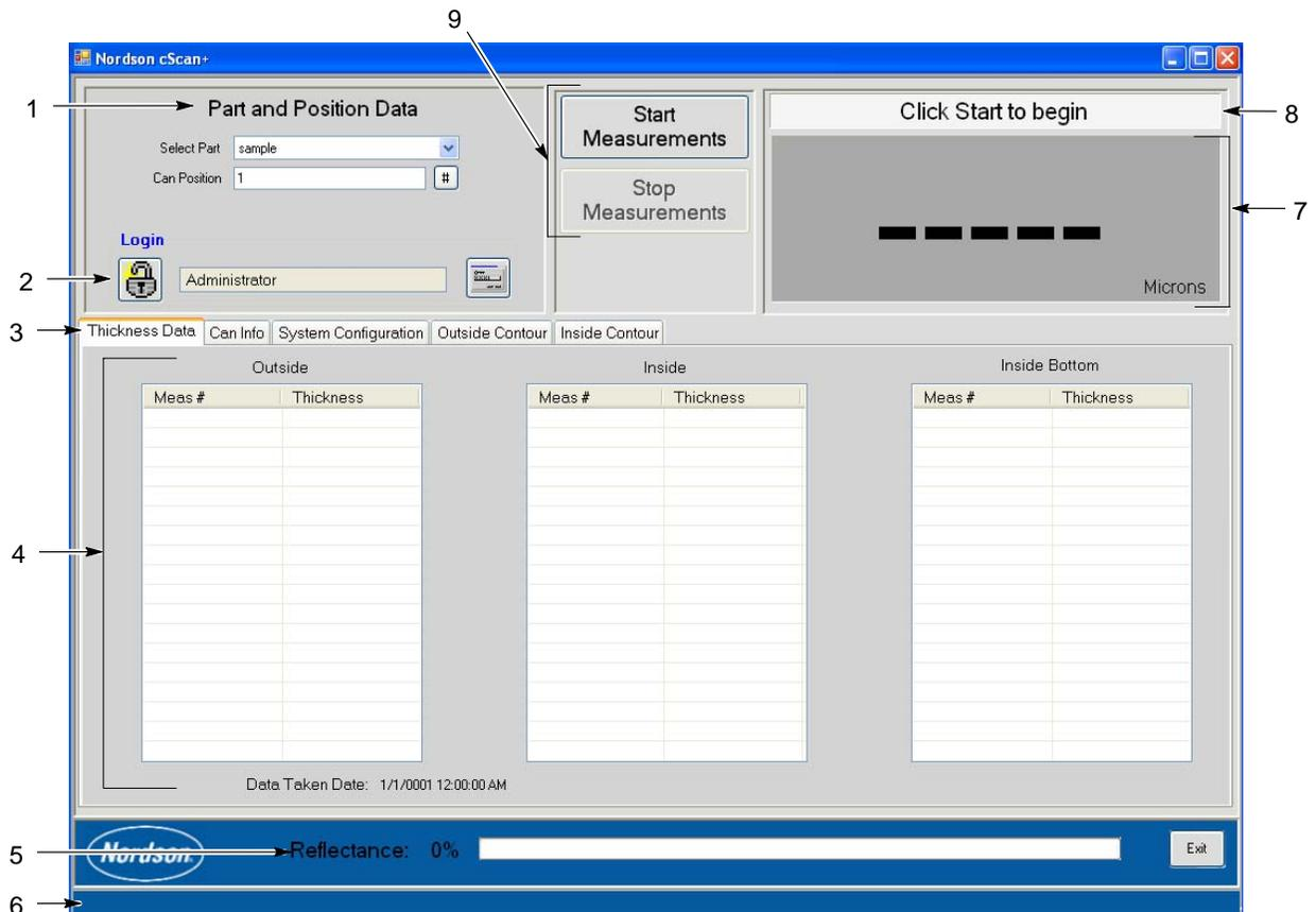
Figure 4 Main Screen for the ACS-1 Software
