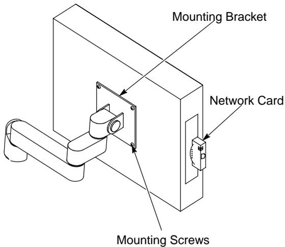
Figure 5 Mount and Network Card Connections for ACS-1 Computer
