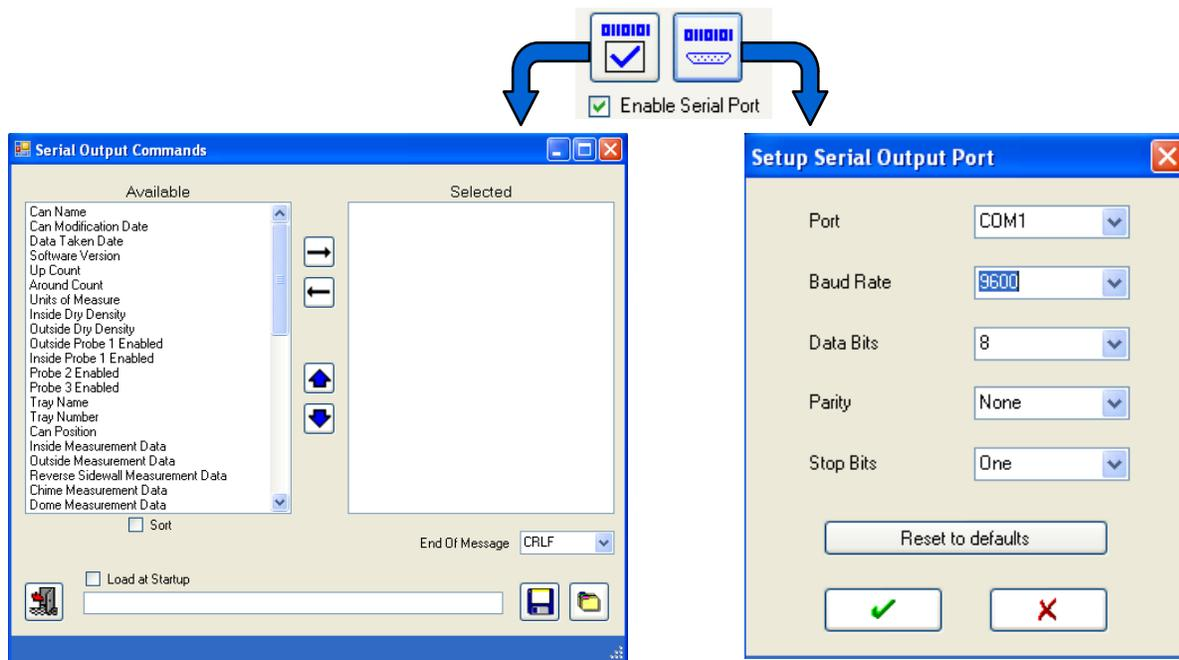
Figure 31 Serial Port Setup
