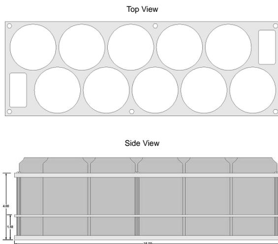
Figure 29 Manual Feed Can Tray
