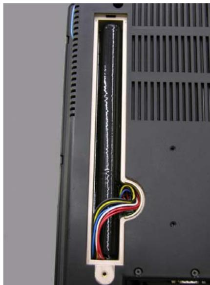
Figure 28 Battery Connected and in Place
