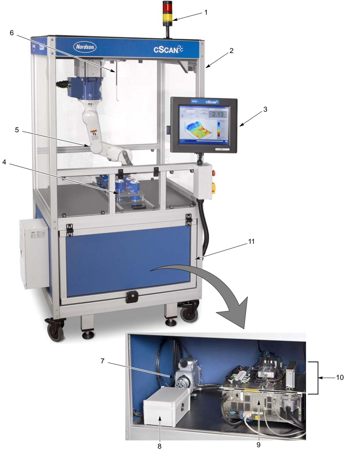
Figure 1 ACS-1 System and Inner Components
