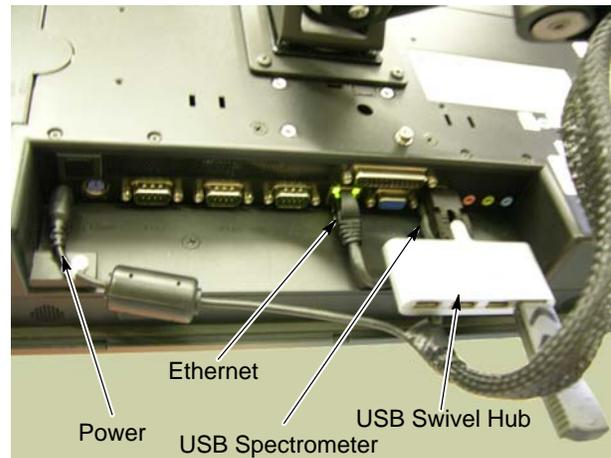
Figure 6 Port and USB Connection on Back of ACS-1 Computer
