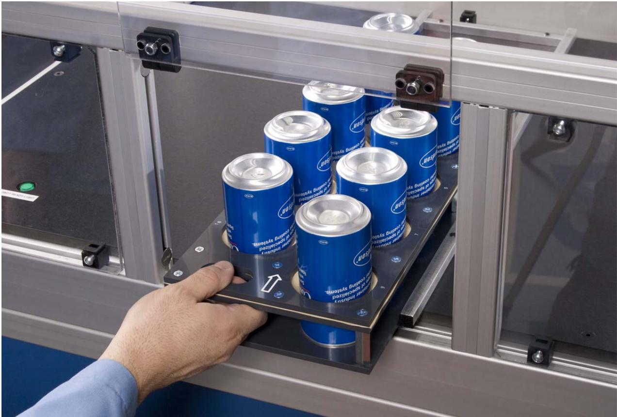
Figure 19 Loading Can Tray into Robot Cell
