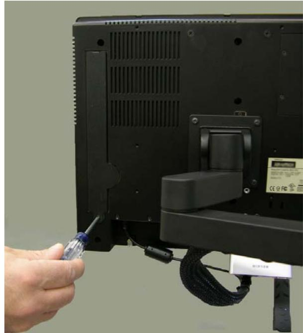
Figure 26 Removing Battery Cover
