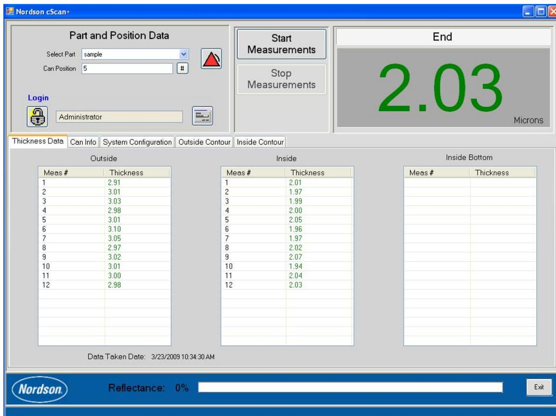
Figure 21 Thickness Data Menu Screen
