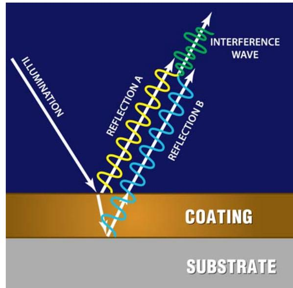
Figure 3 Interference Model
