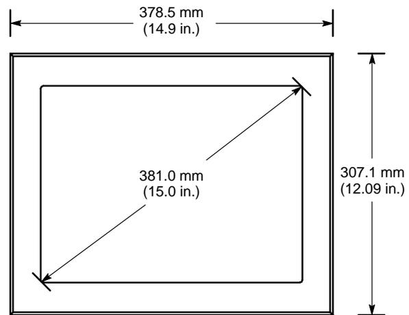
Figure 30 Computer and Monitor Dimensions
