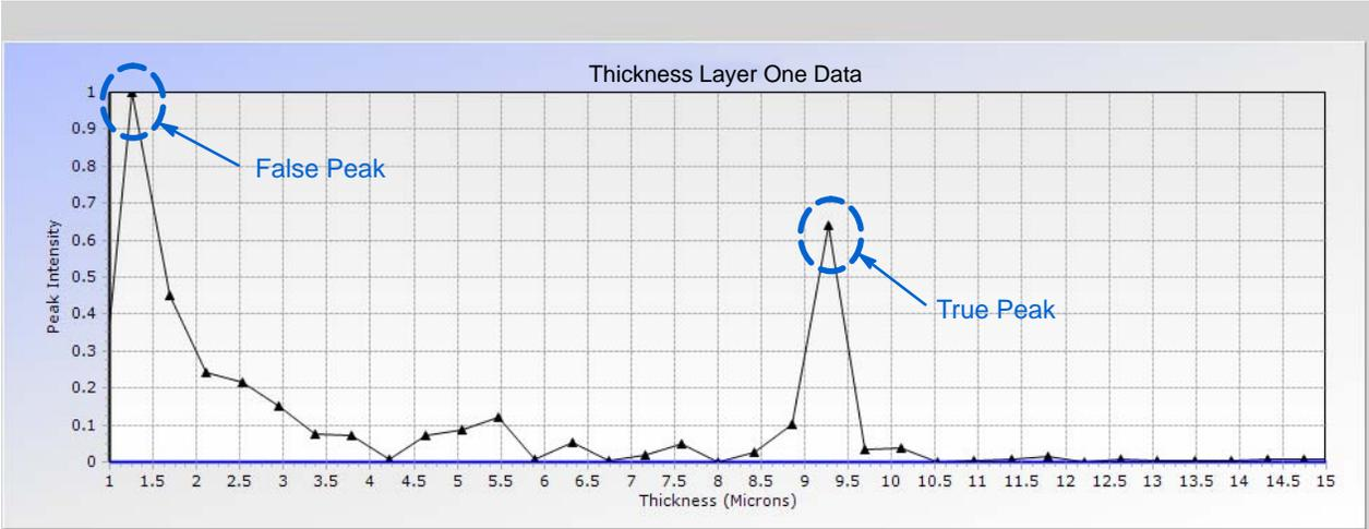
Figure 18 Thickness Data Spectrum with a False Peak and the True Peak
