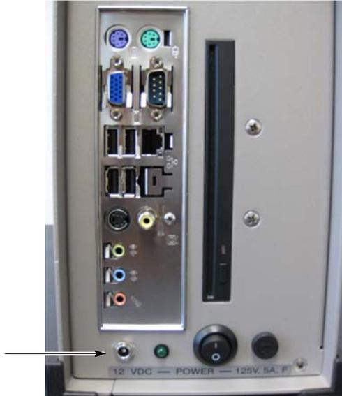
Figure 8 MCS Power Supply Connection
