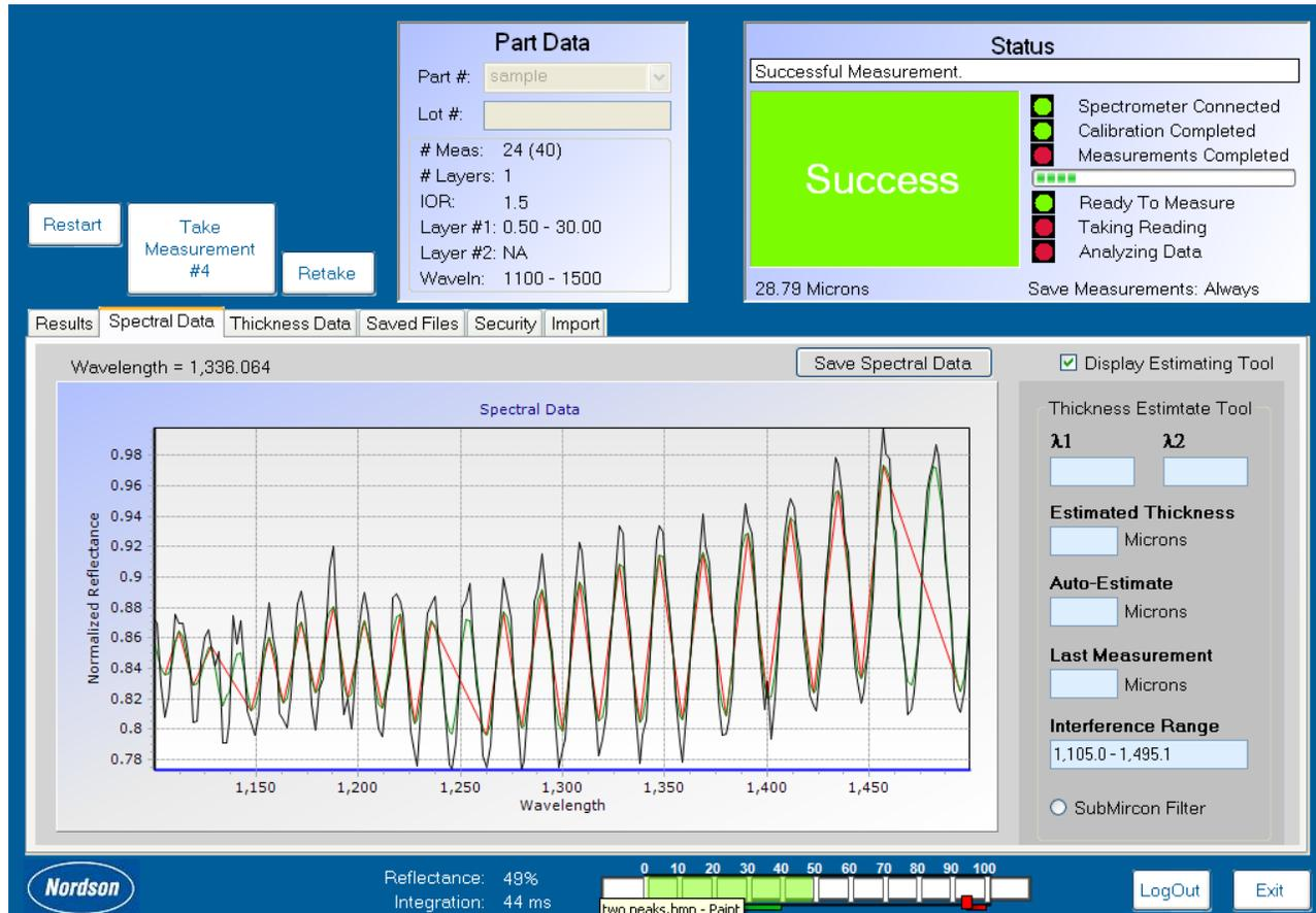
Figure 20 Interference Spectrum Displayed through Spectral Data Tab
