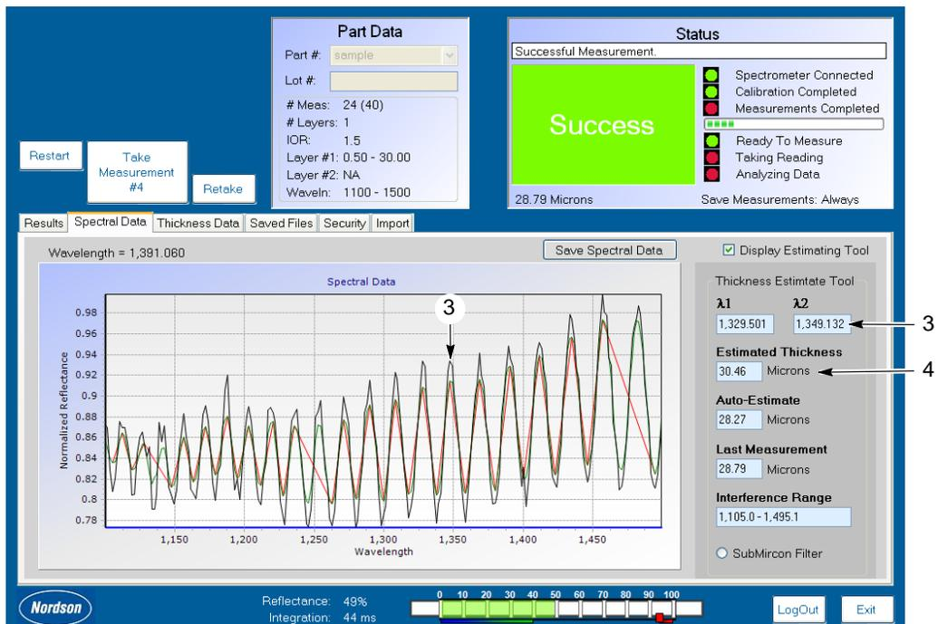
Figure 23 Sine Wave and  $\lambda_2$  Displayed through Spectral Data Tab
