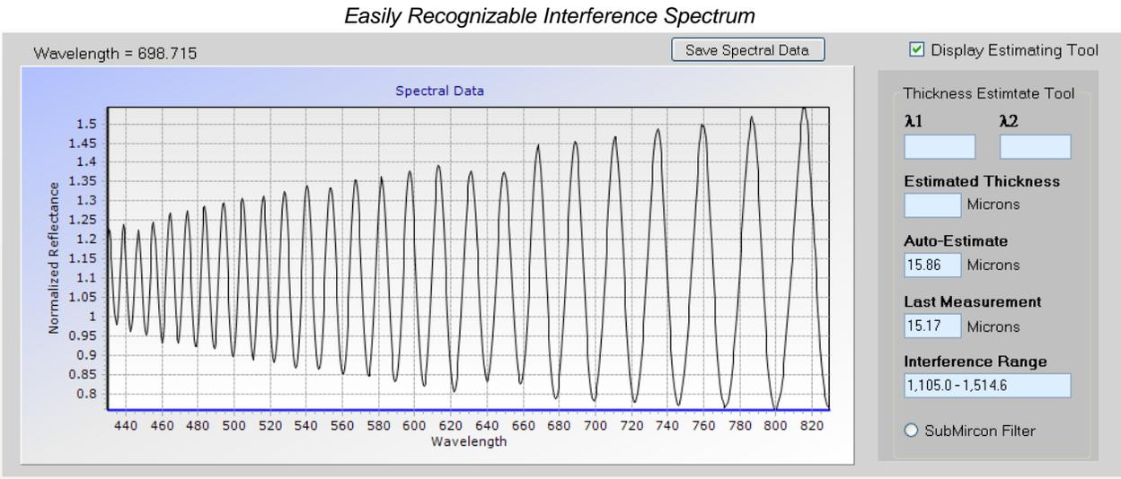
Figure 14 Interference between 430 nm and 830 nm
