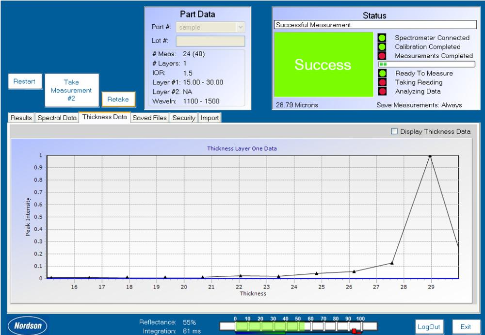
Figure 24 Thickness Data Tab Displayed with True Peak
