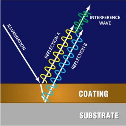
Figure 3 Interference Model
