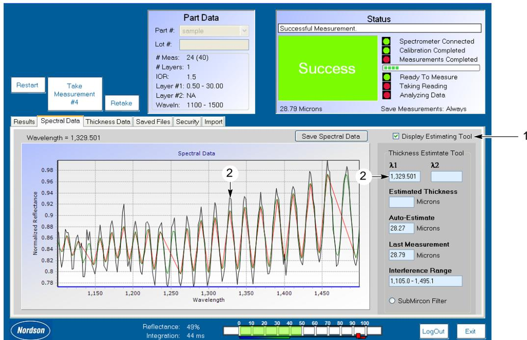
Figure 22 Sine Wave and  $\lambda_1$  Displayed through Spectral Data Tab
