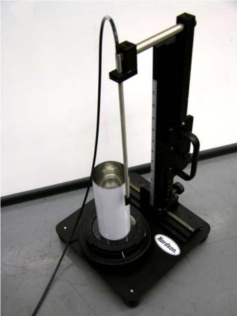
Figure 5 Manual Can Stand with Cable
