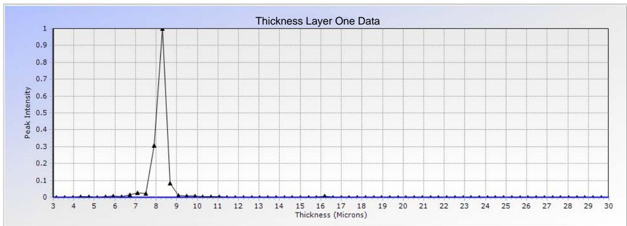
Figure 17 Easily Recognizable Thickness Peak Example
