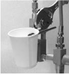
3 Remove the filter element and metal gasket.
