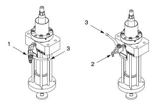
Figure 1 Typical Ball-Valve Bleed Valves
