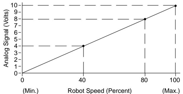
Figure 4 Relationship between Analog Signal #1 and Robot Speed
