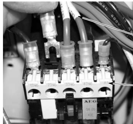
Figure 7 Matching Wire Label to Terminal Label
