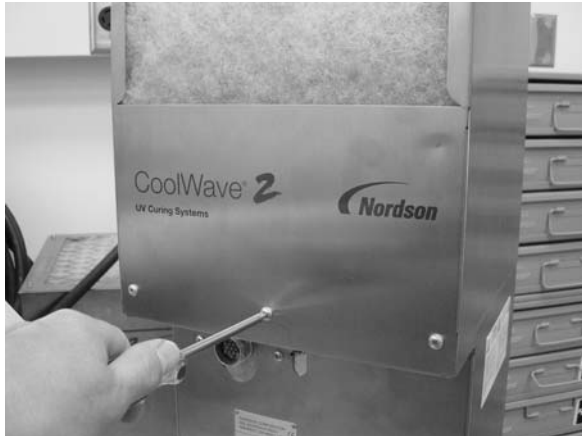
Figure 5-9 Removing Top Blower Cover
