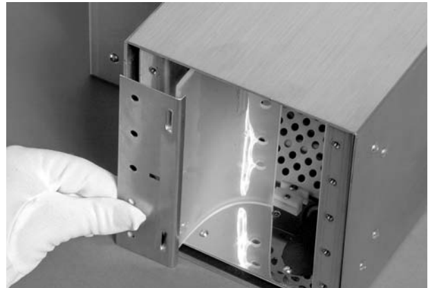
Figure 4-9 Placing the Flood Retaining Bracket
