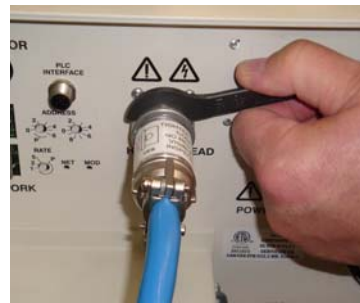
Figure 3-7 Using spanner wrench on screw ring
