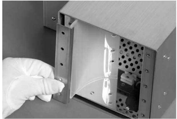
Figure 4-7 Placing the Focus Retaining Bracket
