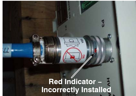
Figure 3-5 Unicable connector partially installed
