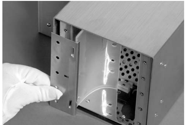
Figure 4-9 Placing the Flood Retaining Bracket
