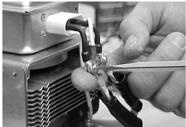
Figure 4-17 Disconnecting Ring Terminals
