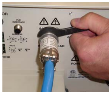
Figure 3-7 Using spanner wrench on screw ring
