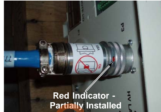
Figure 3-6 Unicable connector partially installed
