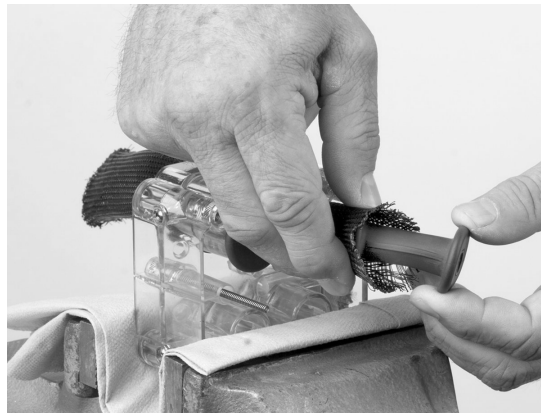
Inserting Pinch Valve into Pump Pinch Valve Tool
