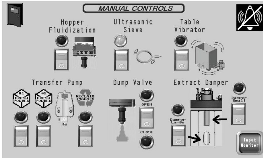
Figure 4-22 Manual Controls Screen
