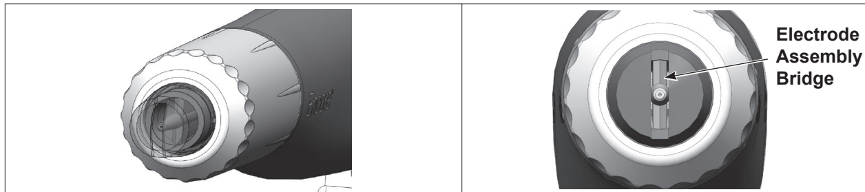
Figure 6 Correct Nozzle Orientation
