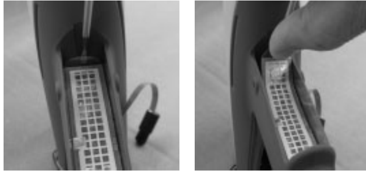
Figure 1-8 Removing the Trigger Switch from the Handle
