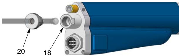
Figure 20 Disconnecting Powder Tubing
