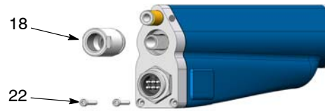
Figure 21 Removing Heat Sink Screws and Lock Nut
