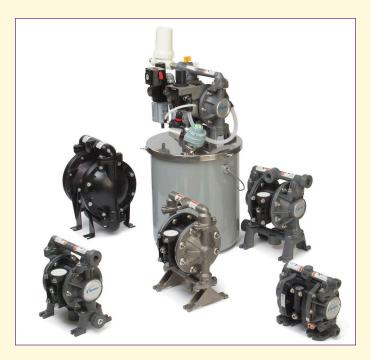
Nordson offers a complete line of liquid diaphragm pumps that are designed to maximize efficiency, compatibility and economy in many applications. Our diaphragm pumps are engineered for low-pressure applications and can handle even the most abrasive or shear-sensitive materials. These self-priming pumps run at variable flow rates controlled by air pressure or fluid back pressure regulation.
