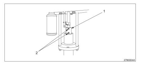
Fig. 2 Removing the Coupling
