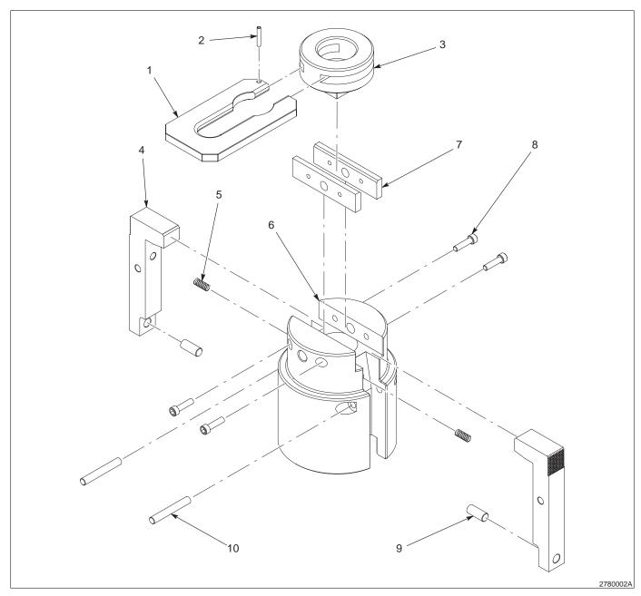
Fig. 4 Rhino Packing Gland Tool Parts
