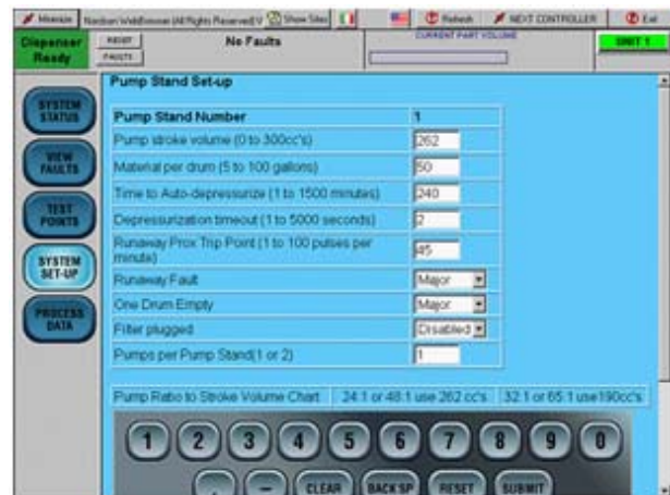
Pump Stand Setup Screen
